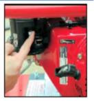
Once the machine is running gently turn the choke to 'off' position
