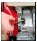
To switch off turn the engine button to the 'off' position.
